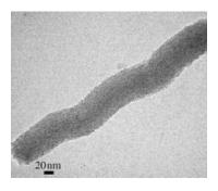
Keep this handy! Periodic mesoporous organosilica-based compounds with chiral channels are prepared by using an achiral fluorinated surfactant (FC-4911) and cetyltrimethylammonium bromide as structure-directing agents. Spiral samples synthesized from 1,4-bis(triethoxysilyl)benzene exhibit structural periodicity and a crystal-like mesoporous wall (see TEM image).
